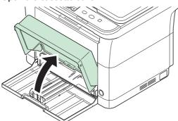
**Note** When using paper that is larger than A4/Letter, remove the cassette cover. Gently press on both the left and right sides of the cassette cover and pull.
